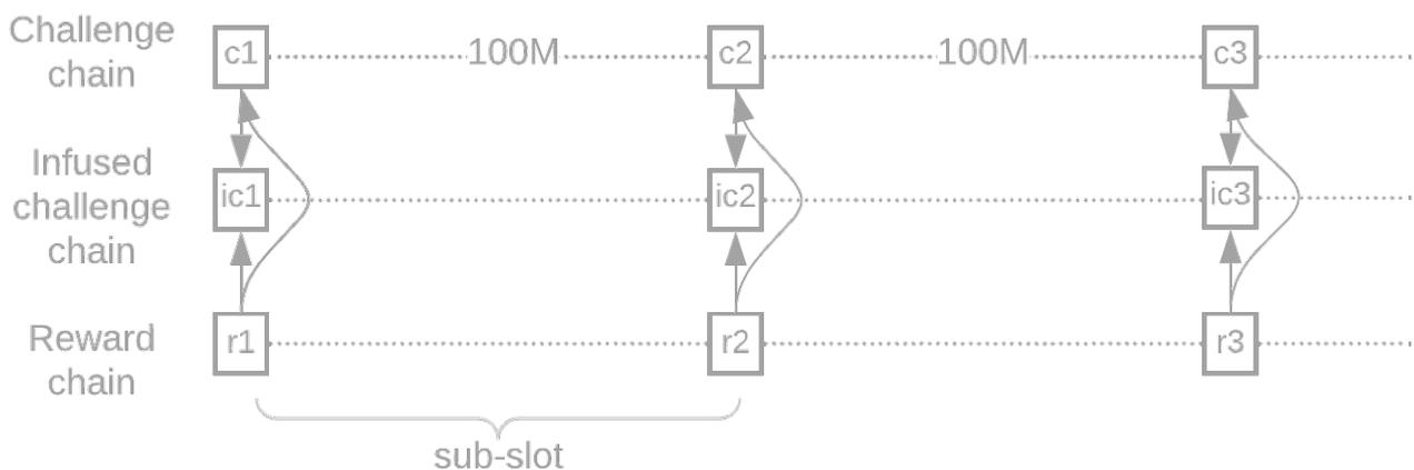
We can see three challenge points, c1, c2, and c3. At these points timelords create challenges (256-bit hashes) which are provided as input to VDFs. Timelords take these hashes, and start computing a VDF on this challenge, for the specified number of iterations. In this example, each slot is 100,000,000 iterations. When the VDF is finished, the timelord publishes the new challenge and the proof of the VDF. An infusion of end-of-slot information happens at the end of each sub-
