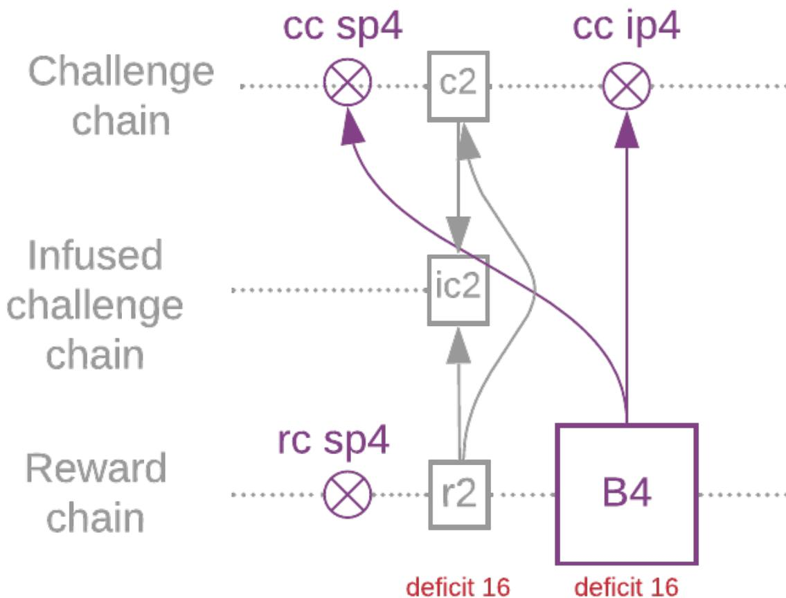
Overflow blocks cannot exist in the first sub-slot of the epoch (since the sub-slot iterations change).
